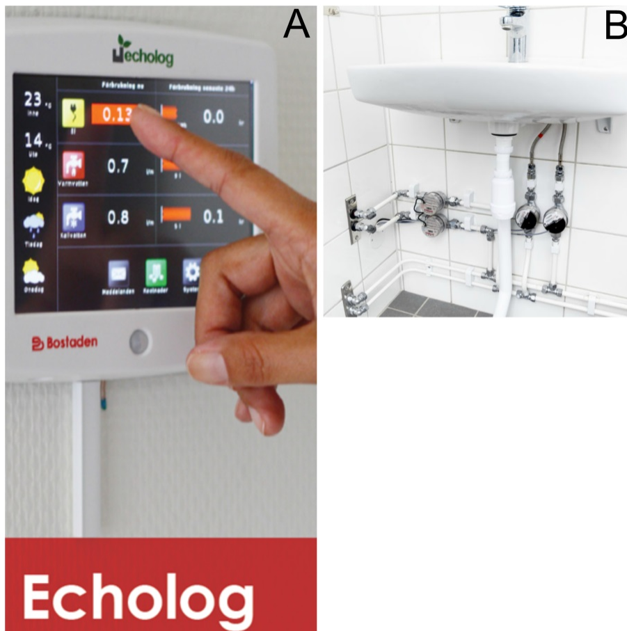
Figure 5.1.: (A) The terminal “Echolog” in all Bostaden’s new apartments shows the consumption of electricity and hot and cold water in real time. The purpose is to help reduce consumption through increased awareness. (B) “Intelligent” equipment as used in the Bostaden pilot study.
